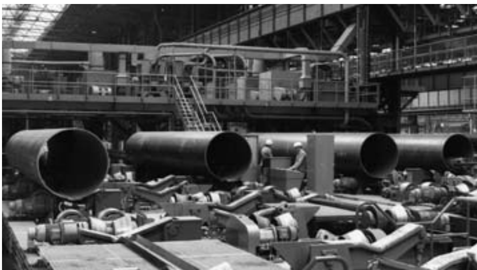
Fig. 62: Longitudinal inside pass submerged-arc welding of large-diameter line pipe (Works photo: EUROPIPE GmbH)
