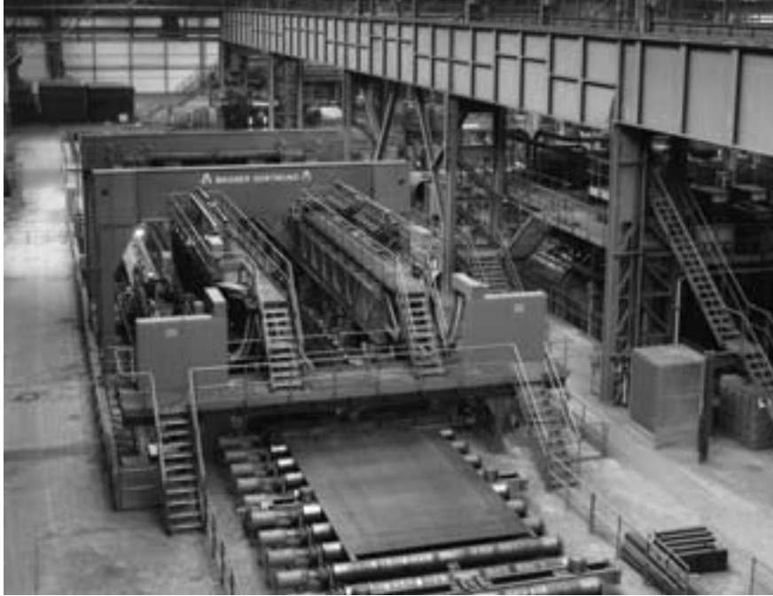
Fig. 57: Planing the two longitudinal edges including the run-in and run-off tabs (Works photo: EUROPIPE GmbH)
