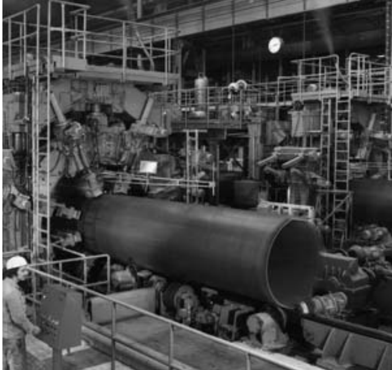
Fig. 61: Continuous longitudinal tack-welding of large-diameter line pipe (Works photo: EUROPIPE GmbH)
