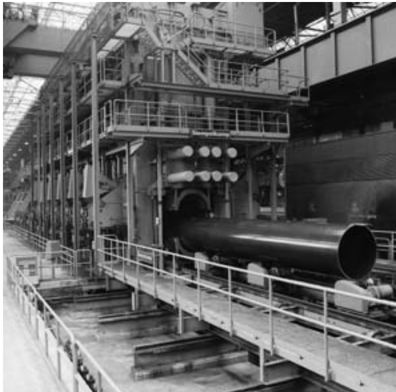
Fig. 60: Completion of the open-seam pipe in the O-ing press (Works photo: EUROPIPE GmbH)
