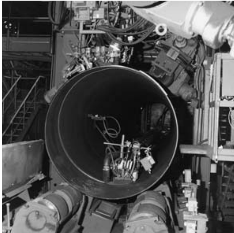
Fig. 70: Computer-controlled combined two-pass submerged-arc pipe welding stand for simultaneous inside and outside weld deposition (Works photo: Salzgitter Großrohre GmbH)
