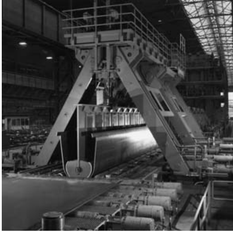
Fig. 59: Forming in the U-ing press (Works photo: EUROPIPE GmbH)
