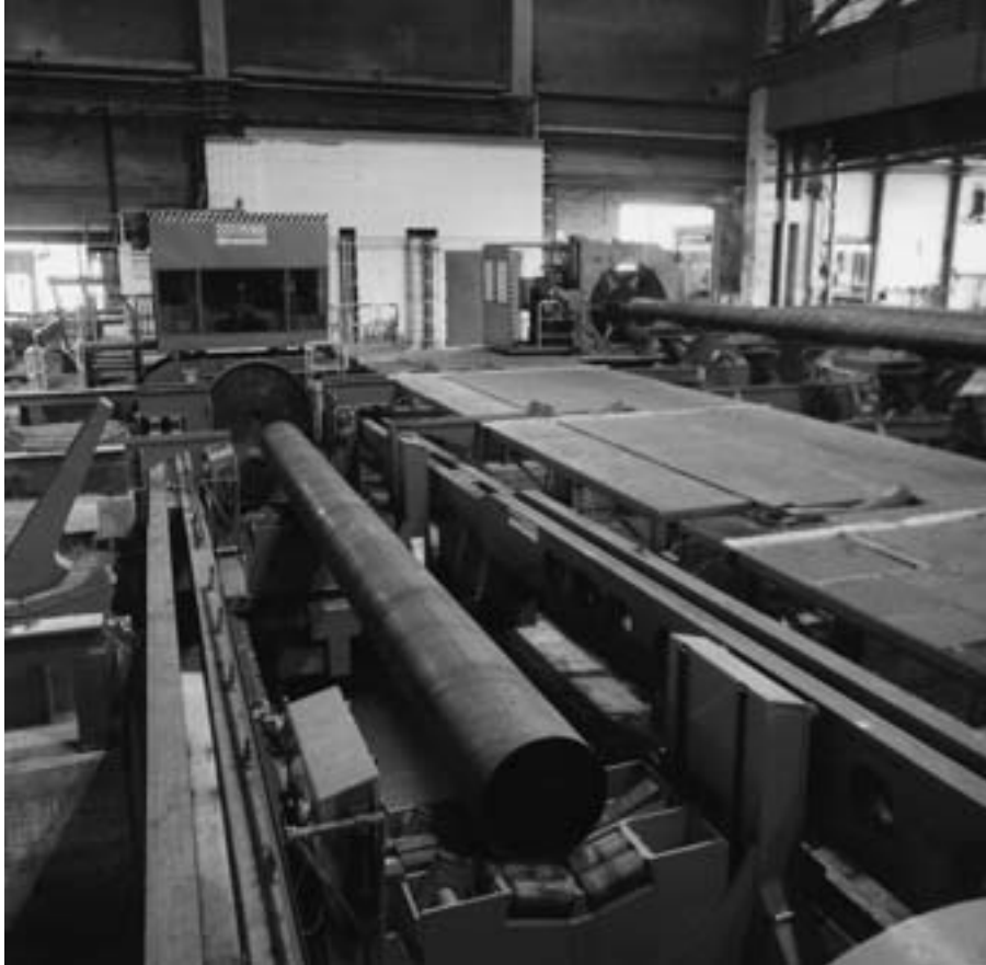
Fig. 67: Hydrostatic testing line with downstream pipe end machining section (Works photo: Salzgitter Großrohre GmbH)
