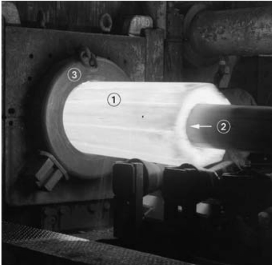
Fig. 25: Inserting the pierced ingot in the drawing press (Works photo: VALLOUREC & MANNESMANN TUBES) 1 Pierced ingot; 2 Mandrel; 3 Drawing die
