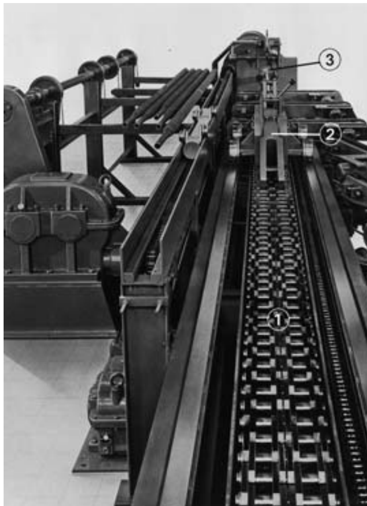
Fig. 33: Draw bench (Works photo: Dahlhaus Iserlohn) 1 Drawing chain; 2 Drawing carriage; 3 Drawing die
