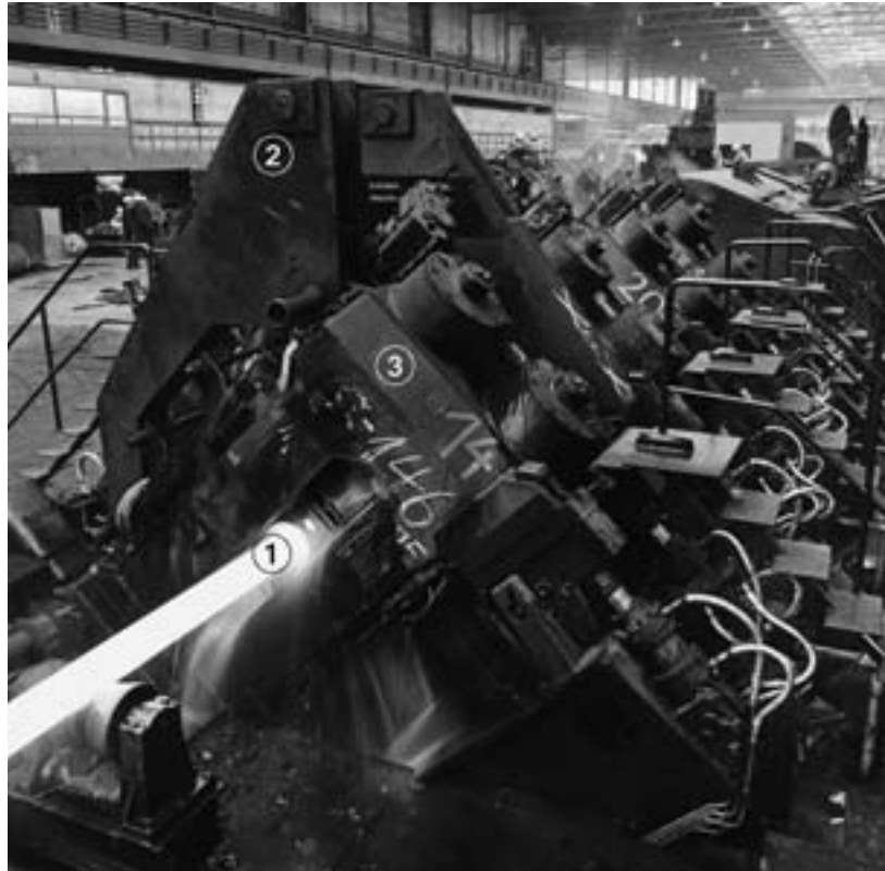
Fig. 16: Continuous mandrel mill (delivery end) (Works photo: VALLOUREC & MANNESMANN TUBES) 1 Pipe; 2 Stand changer; 3 Rolling stand
